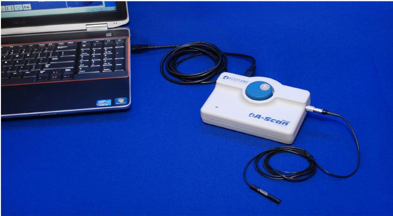
Figure 3.10 - A-Scan Plus Connect Control Unit Connect to a Laptop via USB Cable
